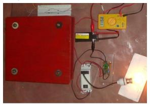
Figure 7: Connected a AC 5W bulb with inverter
